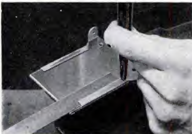
Channels which guide the paper are formed by bending the metal over a suitable shim such as a steel rule
